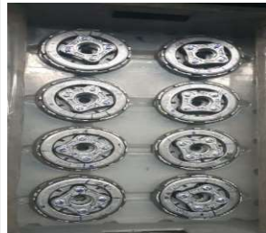
K1E clutch Assy part Polythene Eliminated
