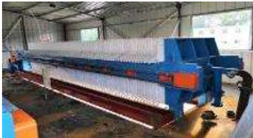
Filter Press for Sludge Handling
